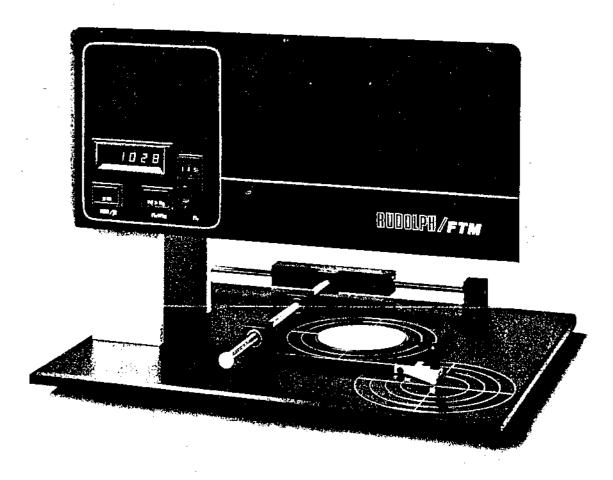
The FTM is the most powerful thin film measuring tool to be introduced in years. The speed, accuracy and simplicity needed for thin film measurements were all designed into the FTM. Oxides, nitrides and photoresists can now be measured in 5 preset positions in far less time then a single point measurement will take using other techniques. This will increase wafer yield through effective and consistent process control.
